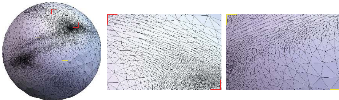
Figure 4: A unit sphere endowed with a metric field derived from the sine-shaped shock function E(x, y, z) = \tanh(\frac{1}{\lambda}(2x - \sin(5y))) + x^3 + xy^2 . \lambda = 0.6 , \rho_0 = 3.0 , r_0 = 0.1 , \gamma_0 = 1.4 , \beta = 2.5 and \delta = 0.3 . The mesh has 18323 vertices and 36642 facets.
