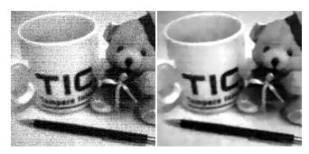
Figure 4: Raw data from cameraphone's CMOS sensor, R channel, 1ms exposure (left), and reconstructed image using the *LPA-ICI* adaptive method with the estimated variance function.
