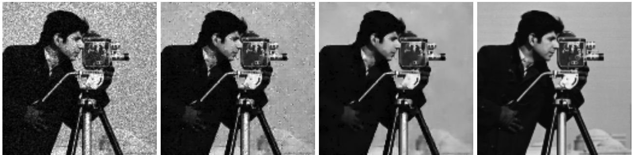
Figure 3. Filtering a fragment of the Cameraman image: (from left to right) noisy data, \chi=60 ( MSE=23.9 ), estimate from the first iteration of the LPA-ICI-AV algorithm ( MSE=7.90 , ISNR=4.81 dB), estimate after the fourth iteration ( MSE=4.36 , ISNR=7.40 dB), and original image.
