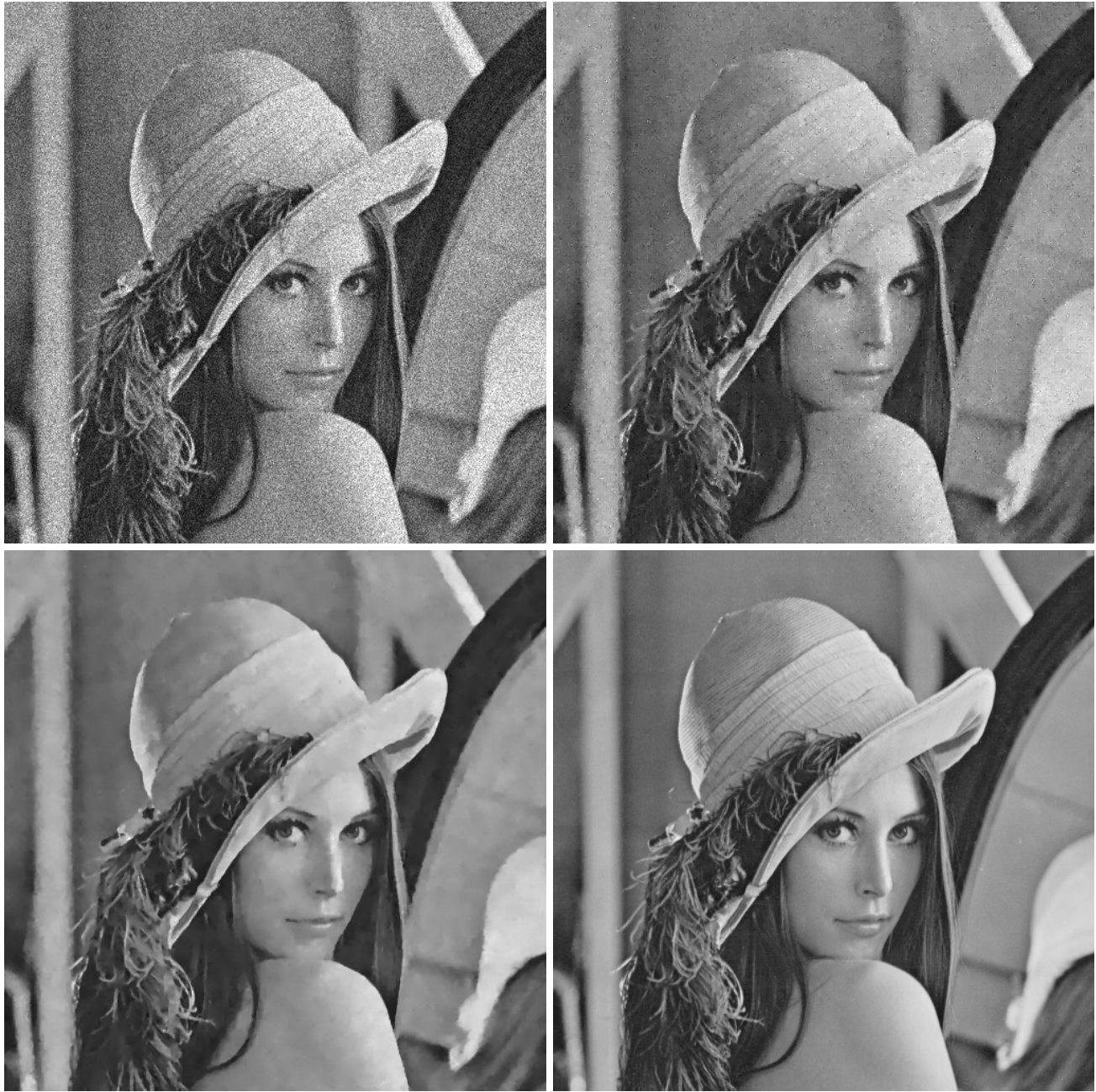
Figure 4. Filtering the Lena image: top row, left - noisy data \chi=60 ( MSE=29.0 , SNR=15.3 dB); top row, right - first iteration of the LPA-ICI-AV algorithm ( MSE=7.07 , ISNR=6.13 dB); second row, left - fourth iteration ( MSE=2.62 , ISNR=10.4 dB); second row, right - original image.
