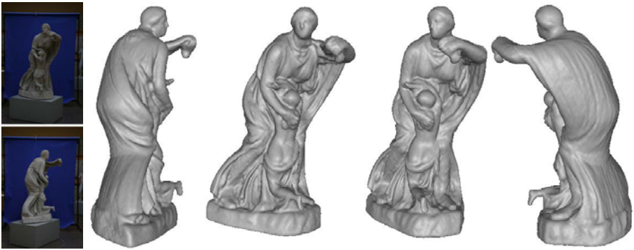
Fig. 6. Niobe sequence. 2 out of 38 input images of resolution 2048 \times 3072 and multiple views of the reconstruction obtained by optimizing the energy model in (5). Note the accurate reconstruction of fine-scale surface details.
