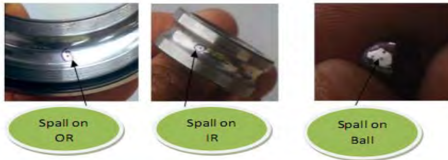
Fig. 3 Localized defect seeded in the bearing elements
