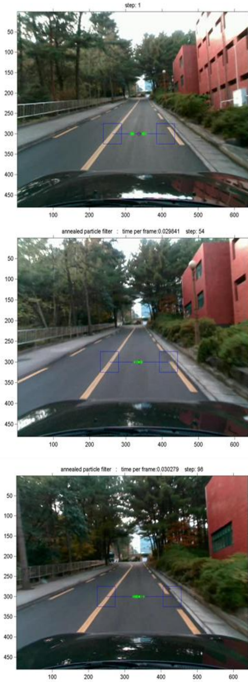
Figure 6. Experimental results. The particle number is 20 ( N=20 ), the annealed layer number is 3 ( M=3 ).
