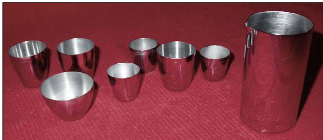
Fig. 7 Chemically stable platinum crucibles. (The red coloration is a reflection of the background.)
