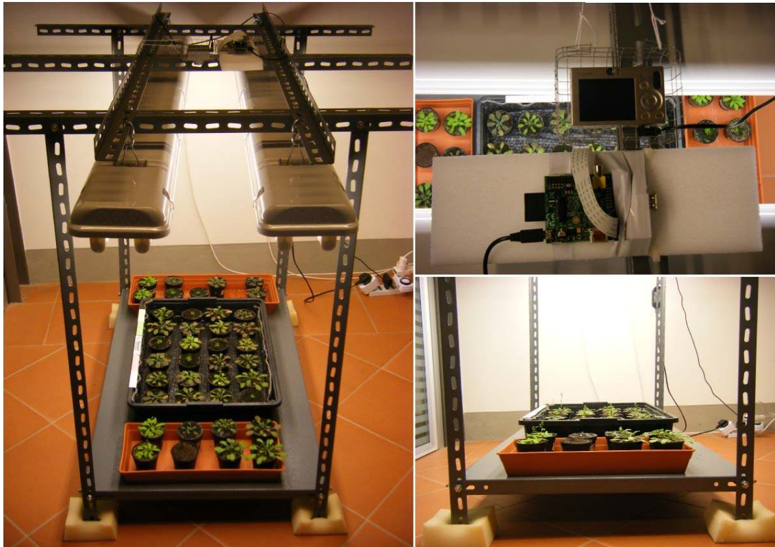
Figure 1: Acquisition setup for ‘Ara2012’ and ‘Ara2013’ datasets, from which ‘A1’ and ‘A2’ datasets were obtained.
