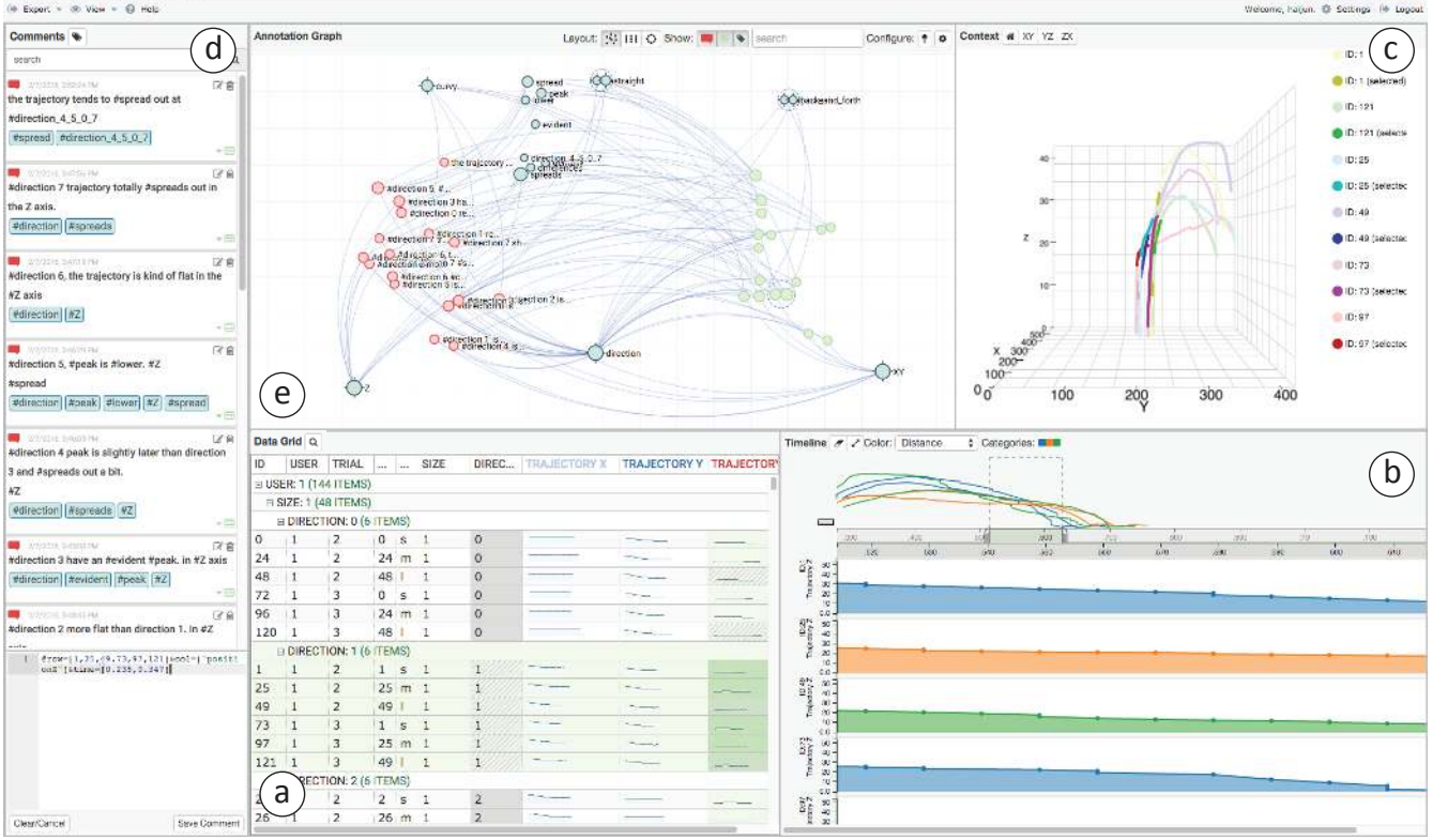
Fig. 3. The front-end interface of the C8 data annotation system: a) Grid View, b) Timeline View, c) Context View, d) Comments View, and e) Annotation Graph View. This particular snapshot features the use of C8 to analyze the results of an HCI user study that records participants pointing at a target on a tabletop display with different experimental conditions.
