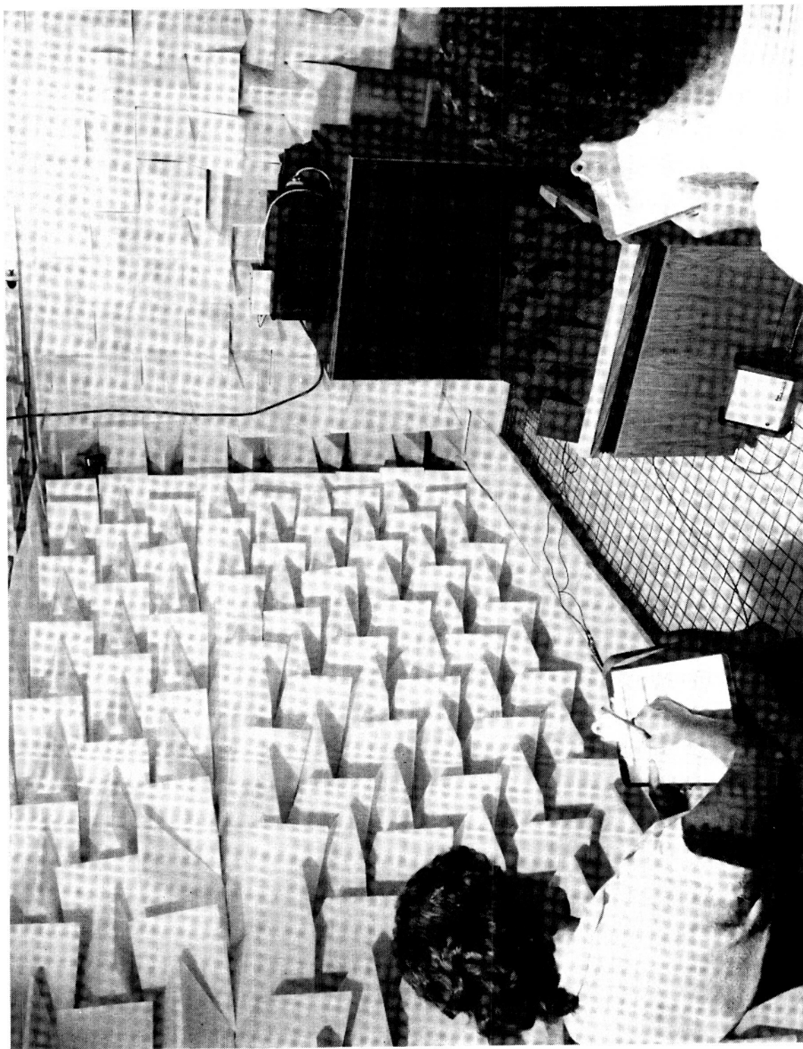
Figure 3. Subjects in Anechoic Listening Room in the Langley Aircraft Noise Reduction Laboratory.
