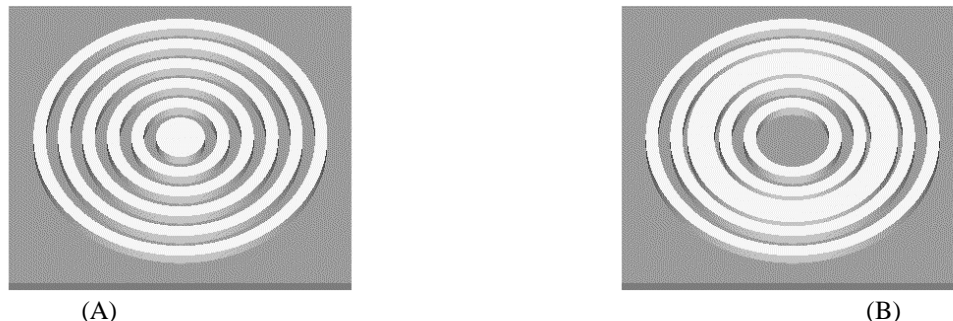
Figure 1. An illustration of A) a Bragg disk resonator; B) an annular Bragg resonator structure.
