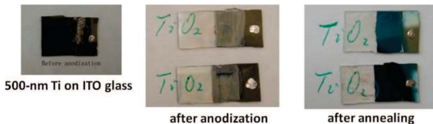
Figure 7. Digital images of 500 nm thick Ti coated ITO glass before anodization (left panel), after anodization (center panel), and after thermal annealing (right panel).
