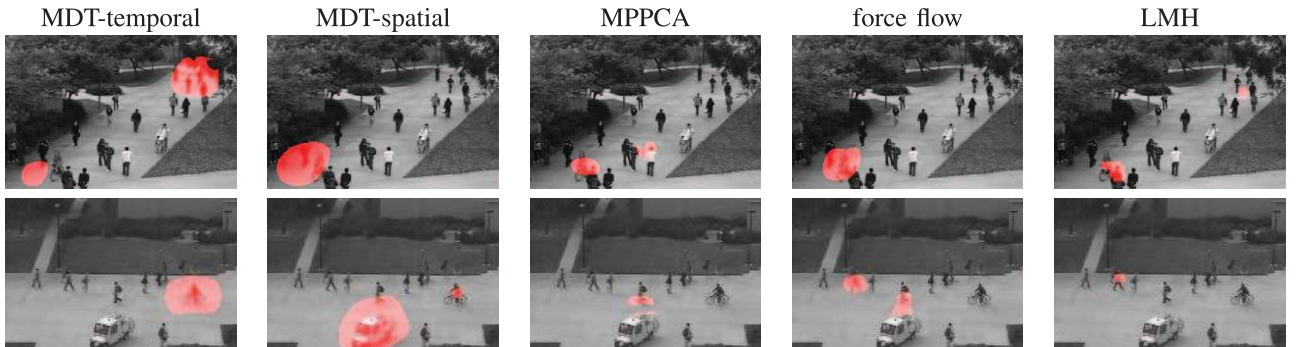
Fig. 6. Anomaly predictions of temporal MDT, spatial MDT, MPPCA, force flow, and LMH (from left to right). Red regions are abnormal pixels. All predictions generated with thresholds such that the different approaches have similar FPR under frame-level protocol (these settings apply to all the subsequent figures unless otherwise stated).
