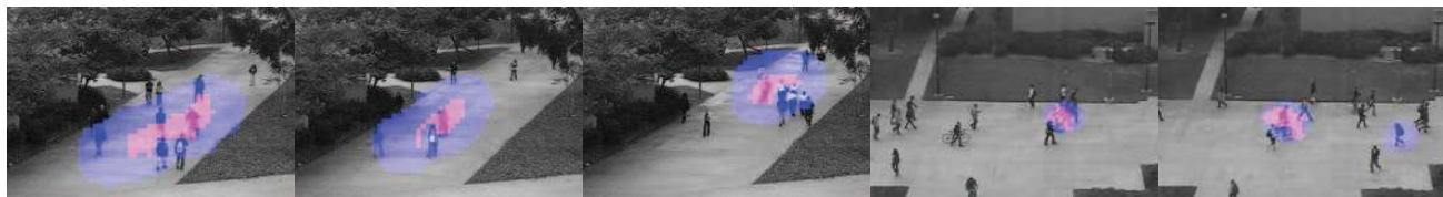
Fig. 7. Examples of anomaly localization with Gaussian smoothing (in blue) and CRF filter (in red). The latter predicts more accurately the spatiotemporal support of anomalies in crowded regions, where occlusion is prevalent.
