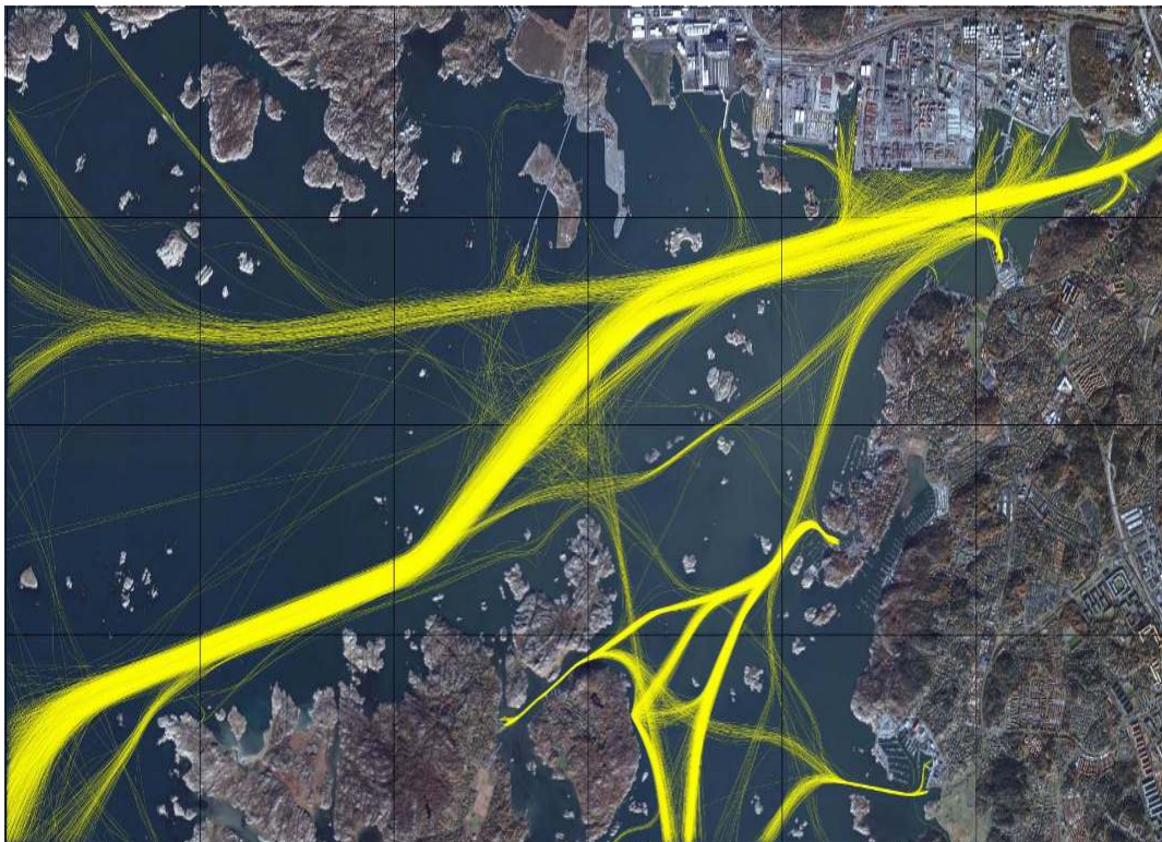
Figure 2: Plot of vessel trajectories extracted from the AIS-dataset covering an area outside the harbor of Gothenburg 4 located in the upper right corner. The grid of size 6x4 used during the experiment is overlaid, where each cell is approximately quadratic with length 2 km
