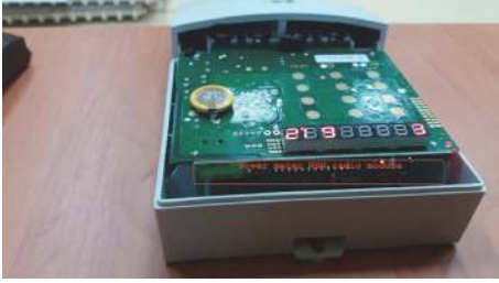
FIGURE 4: Opened power meter with signed WSN communication radio module.
