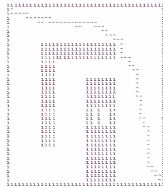
Fig. 3. The Optimal path found by ACO (with obstacles) in a 40X40 grid network
