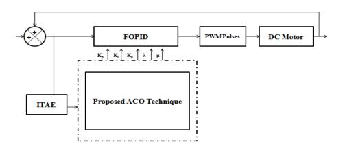
Figure 4 FOPID controller with Proposed Method
