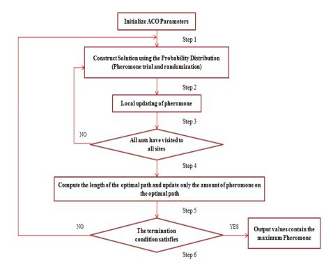
Figure 3 Flow Chart of Ant Colony Optimization technique
