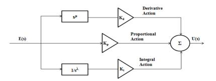
Figure 2 Fractional Order PID controller
