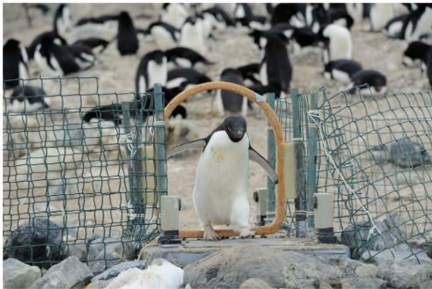
Figure 2. Adélie penguins are identified and weighed each time they cross the automated weighbridge on their way to/from the sea. Picture from David Grémillet. doi:10.1371/journal.pone.0085291.g002
