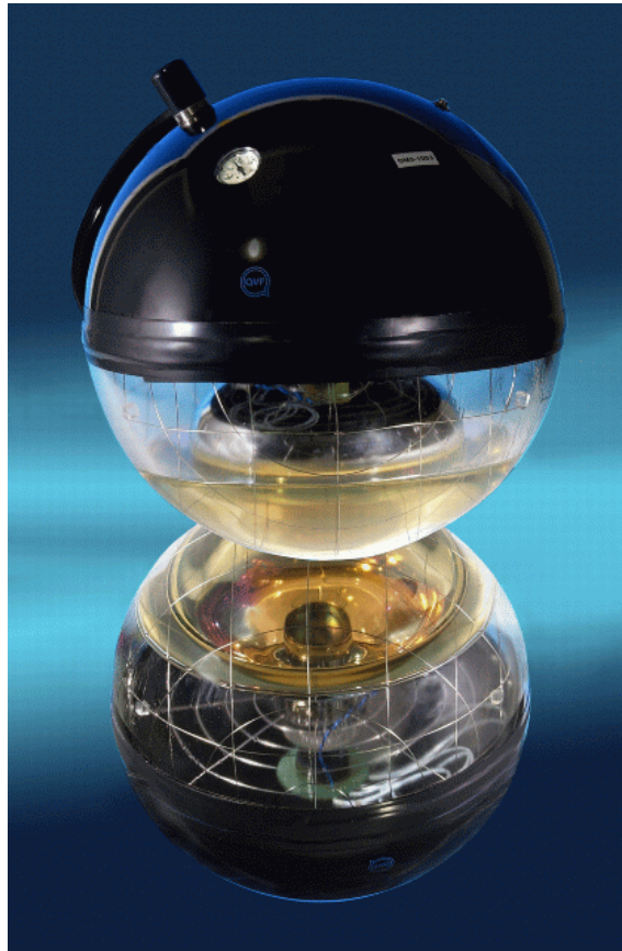
Figure 7: Photograph of an optical module. It is positioned on a mirror to better show the full assembly.
