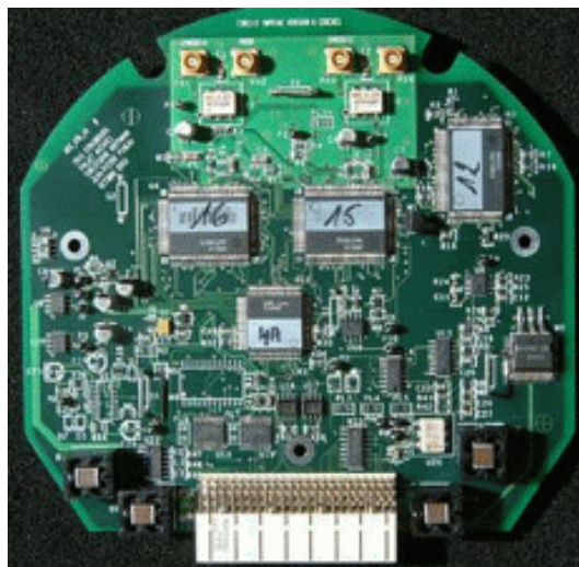
Figure 10: The ARS_MB board with the 2 ARSs (labelled 16 and 15). The 3 rd one (top right, labelled 12) is foreseen for trigger purposes.
