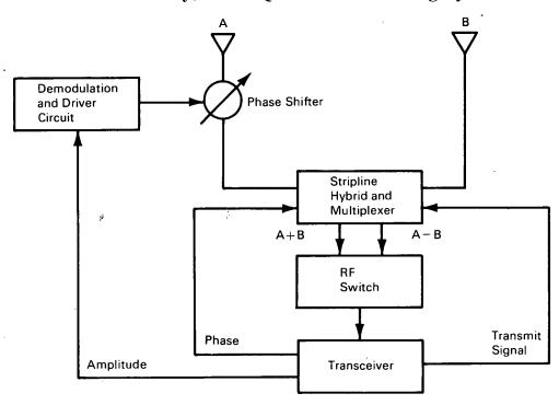
An antenna-array, phase-quadrature tracking system automatically adjusts the phase relationship between the input signals appearing on two widely-spaced parallel-connected antenna elements in the array. An optimum signal is delivered to a transceiver in the control system when a quadrature-phase relationship is achieved between the two input signals.
