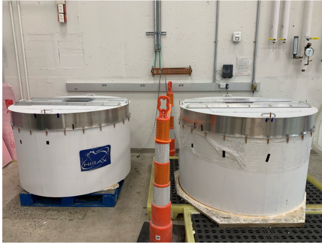
Figure 14. Left: Cavity extenders of 15 cm in length were constructed for the Y-factor system, in order to evaluate the impact of reflections and provide the capability to measure larger antennas. Right: (Top plot) Y-factor measurements of the active HIRAX antenna with both a raised lid and a lowered nitrogen level as compared with the full nitrogen level measurement. Shaded regions indicate measurement uncertainty. These measurements reveal a noise temperature profile that is overall consistent with original cavity measurements in level but differs in feature location. (Bottom plot) Y-factor measurements of the active HIRAX antenna (1) in the raised-lid system using room temperature and liquid nitrogen as hot/cold and (2) mounted to a 3m dish f/d = 0.23 dish, using on-sky measurements with sources in the beam and sources out of the beam as hot/cold.
