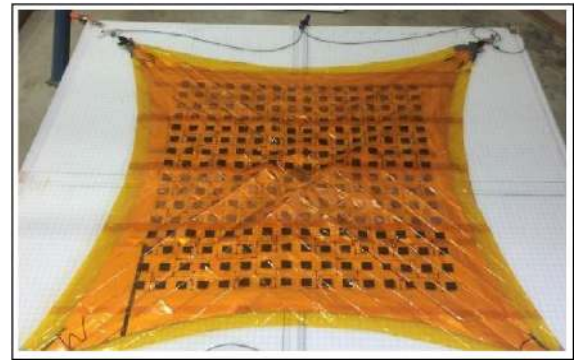
FIGURE 14. S-band deployable patch antenna array for 6U CubeSat [20].
