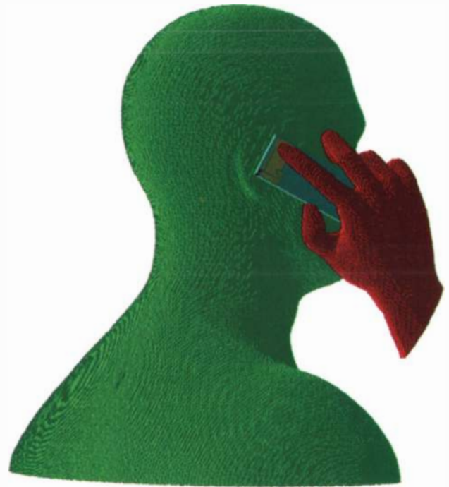
Figure 6. An example of the hand phantom next to the SAM upper-torso phantom.
