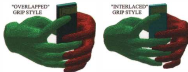
Figure 13. An example of the "overlapped" and "interlaced" grip styles for data-mode hand phantoms.
