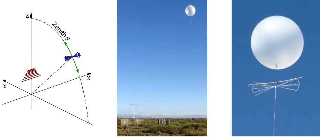
Figure 8: The setup for calibration measurements of the Small Black Spider LPDA at the site of AERA. Left: Sketch of the measurement setup. A calibrated transmitter antenna is moved on a circle around the antenna under test to access different zenith angles. Only the read out plane of the tested antenna is displayed. Middle: A picture of the setup. In the lower left the AERA station used for the calibration measurement is visible. At a distance of \sim 30 m a balloon carries the calibrated transmitter antenna. The position of the transmitter is fixed by a three-legged rope system which provides the movement on the circle and a parallel orientation of the transmitter and receiver antenna. Right: Picture of the calibrated biconical antenna used as transmitter. The biconus has a length of 1.94 m. The antenna is carried by a balloon filled with 5 \text{ m}^3 helium and is fed by a coaxial cable running to the ground. The overall weight lifted by the balloon is \sim 4.5 kg.
