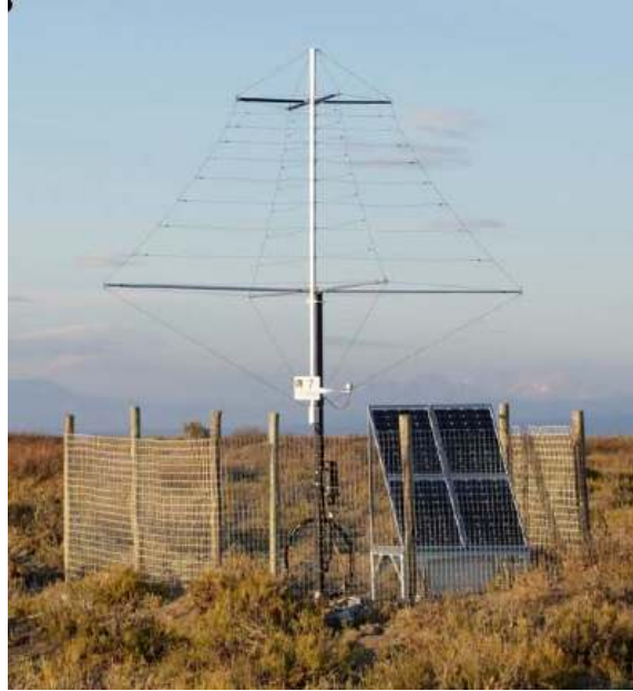
Figure 2: A radio detector station of the first stage of AERA. A logarithmic-periodic dipole antenna, called Small Black Spider, is used as sensor for the radio emission of extensive air showers. The antenna is read out with digital oscilloscopes and a trigger decision on air shower signals is performed by an FPGA. A photovoltaic power system enables autonomous operation of the detector station and supplies the readout electronics, the GPS system used for timing, and the communication system.
