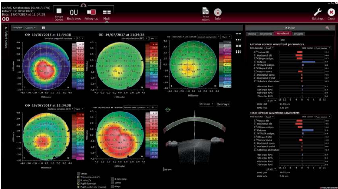
Fig. 13.9 ANTERION Cornea App multiview. Five corneal maps (anterior tangential curvature, anterior elevation, corneal pachymetry, posterior elevation and anterior axial curvature), OCT image and wavefront parameters of a keratoconus eye
