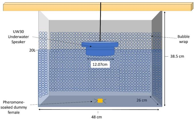
Fig 2. Experimental tank setup with 1) bubble wrap lining three sides of the interior of the tank to reduce sound reverberation, 2) hanging underwater speaker so just speaker is submerged under the water line from a horizontal wooden plank, and 3) pheromone-soaked sponge made to resemble a female crab.
