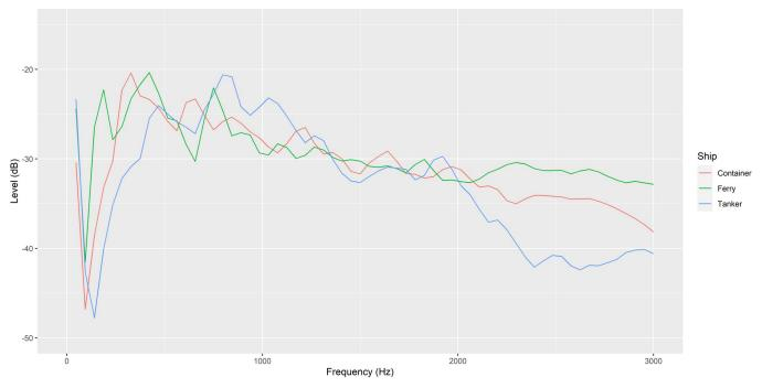
Fig 3. Spectrograph (Hann window, size 1024) showing the average sound profile (amplitude/level and frequency) of the original recording of three ships recorded in UK harbours approximately 200 metres away [17].
