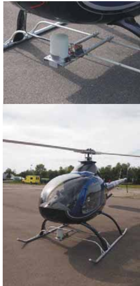
Fig. 10. Installation of anti-collision system on A600 "Talon" helicopter
