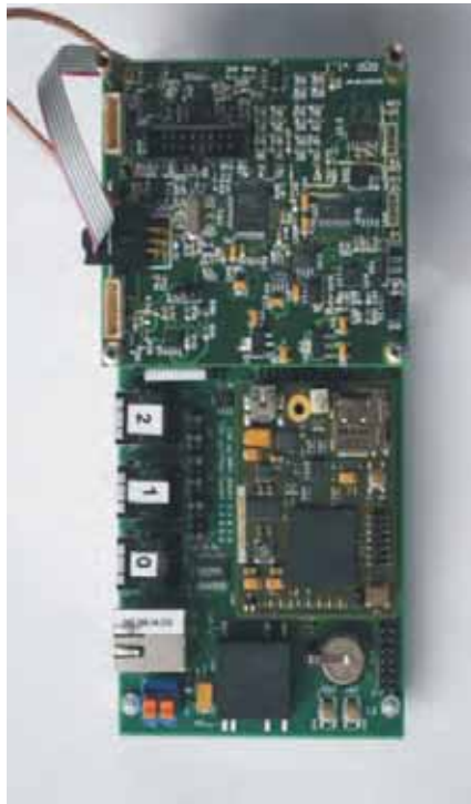
Fig. 9. Micro Computer AXMOD with A/D converter
