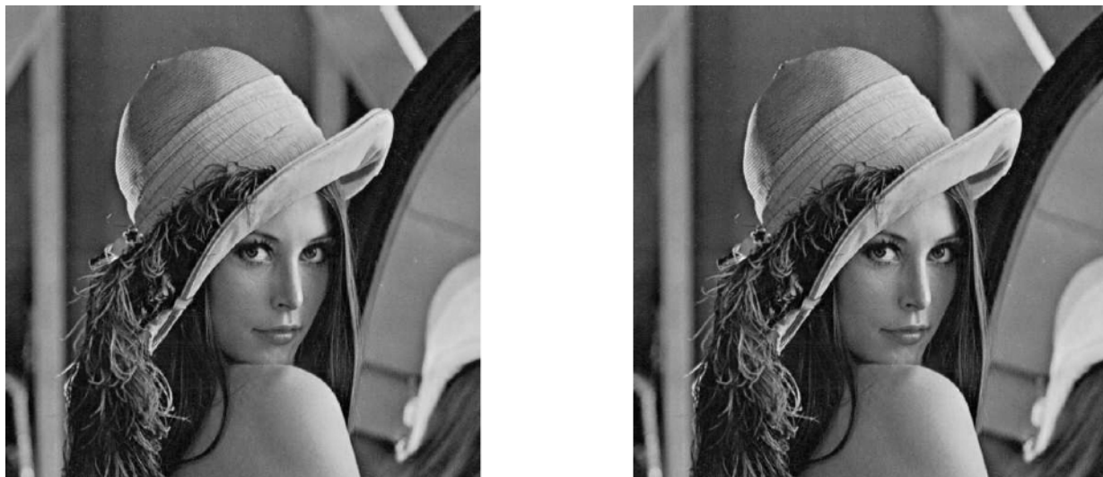
Fig. 8. Left: An image compressed using the SPIHT algorithm at a bit rate of 3 bits per pixel before the use of entropy coding. Right: The same image after anti-forensic dither has been applied to its wavelet coefficients.
