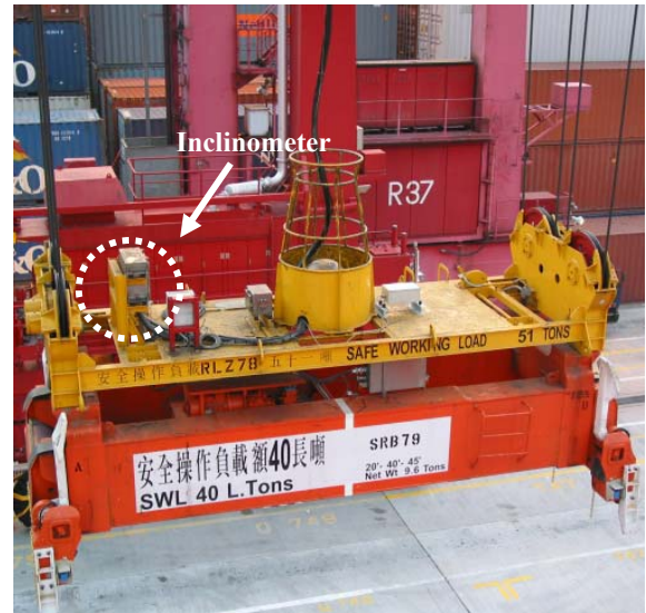
(b) The head block and an inclinometer.
