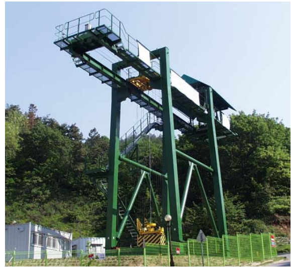
Fig. 7. The pilot crane used in experiment: an RMQC type.
