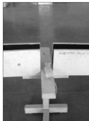
Figure 2: Photograph showing the activity of mice on elevated plus maze. Open arms (16 cm x 16 cm) and two covered arms (16 cm x 5 cm x 12 cm). The arms extended from a central platform (5 cm x 5 cm), and maze was developed to a height of 25 cm from the floor
