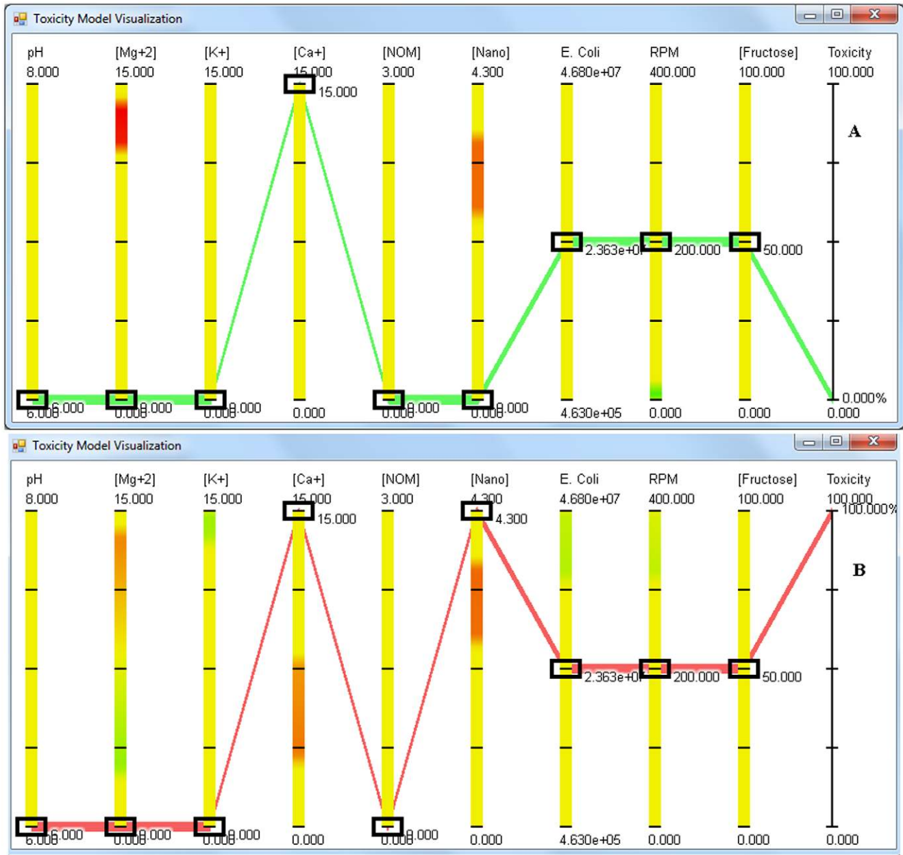
Figure 9. Screen shot of the visualization application showing the effect of calcium salts on the anti-bacterial activity of CeO 2 NPs at a) 0 ppm nanoparticle concentration and b) 4.3 ppm nanoparticle concentration. The concentrations of MgSO 4 , KCl and NOM is set to 0, CaCl 2 and E. coli are at 15 ppm and 2.36 × 10 7 CFU/mL respectively whereas RPM and fructose are set at 200 RPM and 50 ppm respectively. doi:10.1371/journal.pone.0047827.g009
