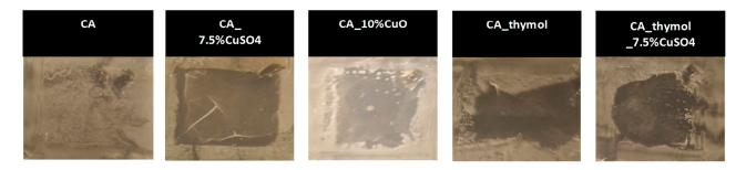
**Figure 3.** Antibacterial activity of filter materials against bacteria *Escherichia coli* and *Staphylococcus aureus*. The filter materials were removed for the images to demonstrate the bacteria-free area under the materials.
