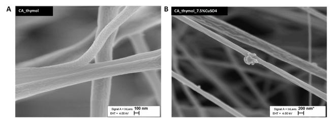
**Figure 2.** Morphological characteristics by SEM imaging for electrospun CA filter mats comprising thymol (**A**) and CuSO<sub>4</sub> (**B**) as additives, showing the texture change on the surface.
