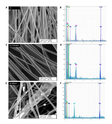
**Figure 1.** Morphological characteristics by SEM imaging for electrospun CA filter mats (panels **A**,**C**,**E**) and EDX analysis of the mats (panels **B**,**D**,**F**). Please refer to the different scales on the *y*-axis.
