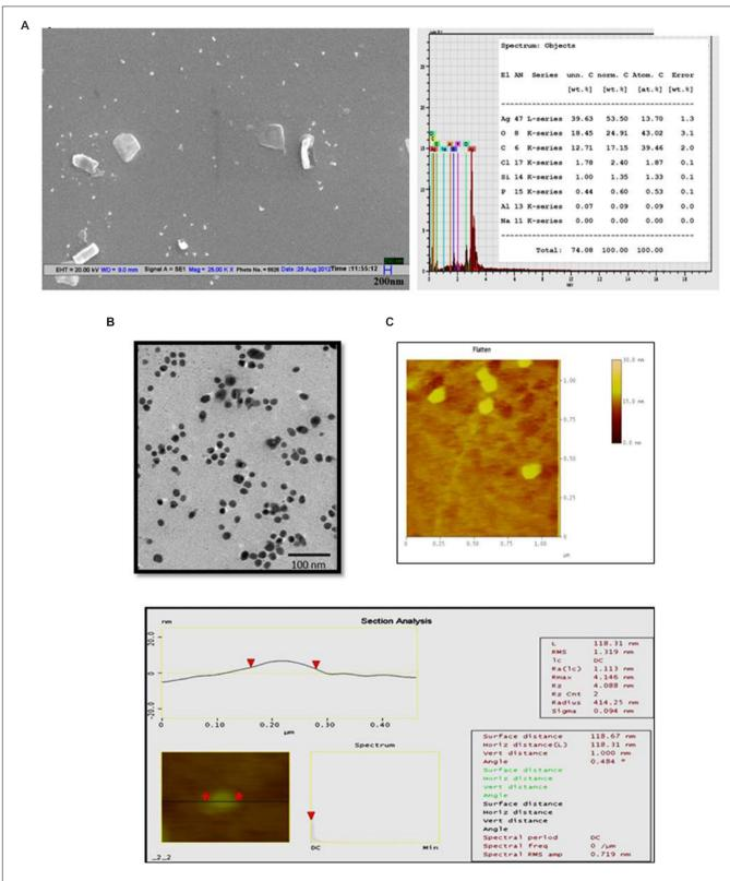
FIGURE 1 | Microscopic analysis of green synthesized Jc-AgNps. (A) Left: SEM image of Jc-AgNps showing variation in sizes (50–100 nm); Right: energy-dispersive X-ray (EDX) patterns of Jc-AgNps showing strong signals of silver (20 kV), (B) Transmission electron microscopic images of Jc-AgNps. Images were taken at 200 kV on a carbon-coated Cu grid, (C) AFM image showing root mean square along with major statistical parameters of Jc-AgNps.
