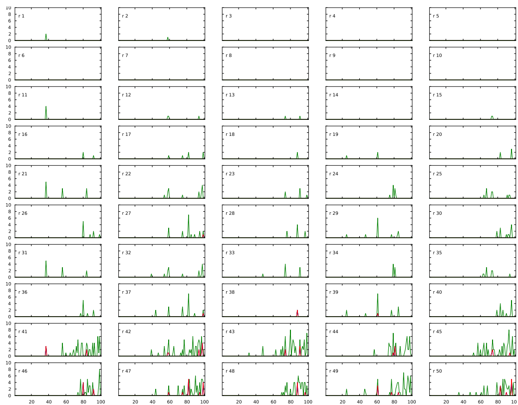
Figure 57: Number of ten-day periods that the water levels in the IJsselmeer are above threshold values in the winter half year for all 50 climate realisations in case a additional pump capacity of 500 \text{ m}^3/\text{s} is implemented at the Afsluitdijk. Green 0.1-0.3 m MSL and > 0.3 \text{ m MSL}
