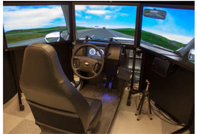
Fig. 2. NADS MiniSim driving simulator.
