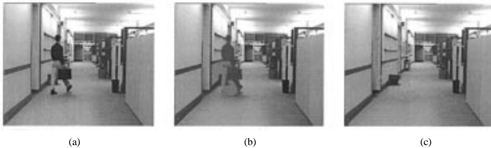
Fig. 21. (a) Original image. Example of restitution (b) without compensation and (c) with motion compensation in the case of motion connected operators.
