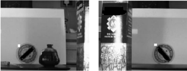
Fig. 14. Detection results for beer coaster under varying pose and illumination. The average number of detectors per pixel was 1.15.
