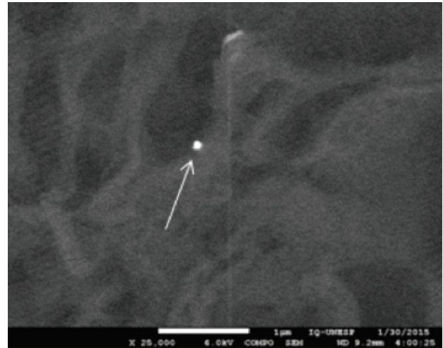
Figure 2 - Backscattered SEM image of Ag2 specimen, showing presence of silver particles (arrow).
