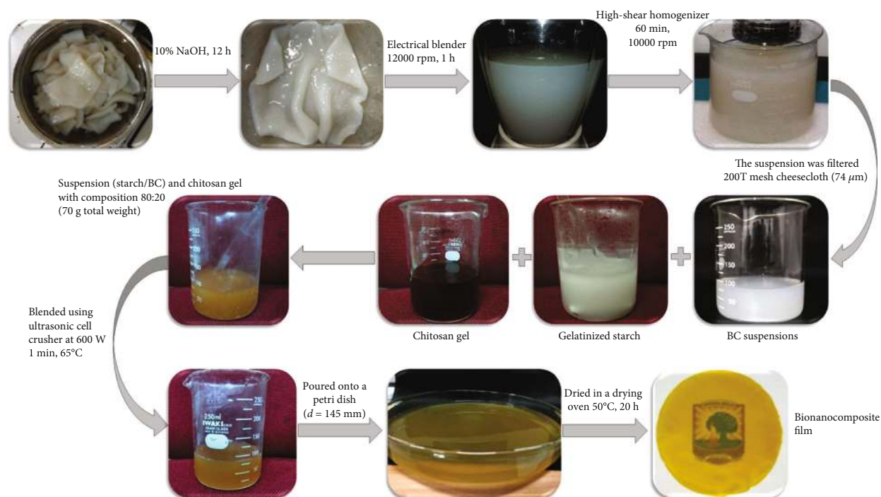
FIGURE 1: Steps of sample preparations for biocomposite.
