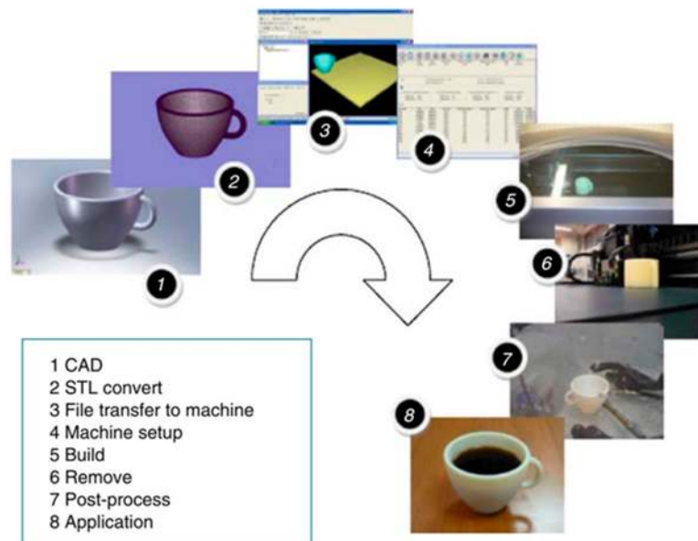
Figure 1. Steps involved in the fabrication of a cup by additive manufacturing (AM). Reproduced with permission from Ref. [1].
