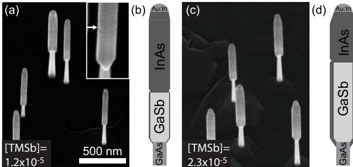
Figure 5.1: *SEM images at 30° tilt angle of GaSb/InAsSb nanowires grown on GaAs stems using a TMSb molar fraction of (a)  $1.2 \times 10^{-5}$  and (c)  $2.3 \times 10^{-5}$  during the GaSb growth step, respectively. The arrow in the inset indicates the occurrence of additional faceting near the GaSb/InAsSb heterojunction. The schematic images (b,d) clarifies the structural differences between the nanowires in a and c, respectively.*
