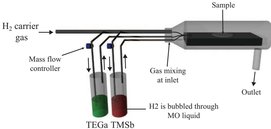
Figure 2.4: *Schematic illustration of a MOVPE reactor for GaSb growth. H<sub>2</sub> gas is bubbled through containers of growth precursors, which are then transported into the heated growth chamber where the sample is located and the epitaxial growth occurs.*
