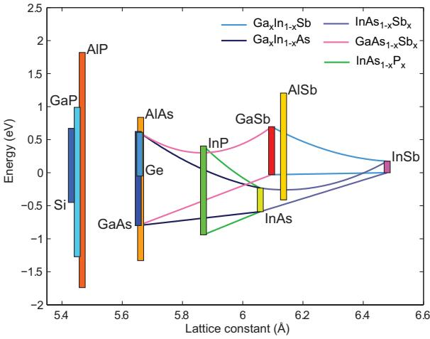
Figure 3.1: *Band gaps and band alignment of the group IV and selected III-V binary and ternary semiconductors plotted as function of the cubic lattice parameter. The lines correspond to the valence band and conduction band positions for ternary alloys over their whole composition range (Data from Ref. [23]).*
