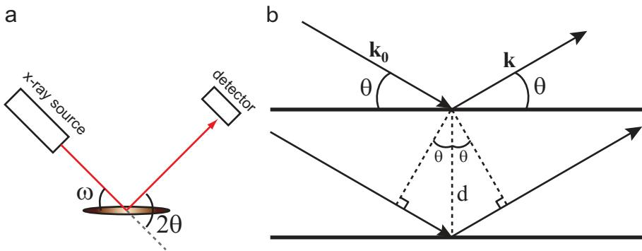
Figure 2.5: (a) A simplified schematic of an HRXRD setup. (b) X-rays reflected off two consecutive crystal planes with incidence and exit angles  $\theta$  relative to the planes. Note that  $\omega = \theta$  is only true if the normal of the diffraction planes is parallel to the sample normal. This is generally not the case.
