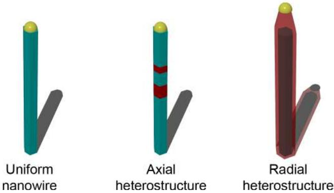
Figure 4.1: *Examples of possible nanowire structures. It is possible to include either axial or radial heterostructures into the nanowire crystal. Because of the small diameters of nanowire, lattice-matching requirements are relaxed.*
