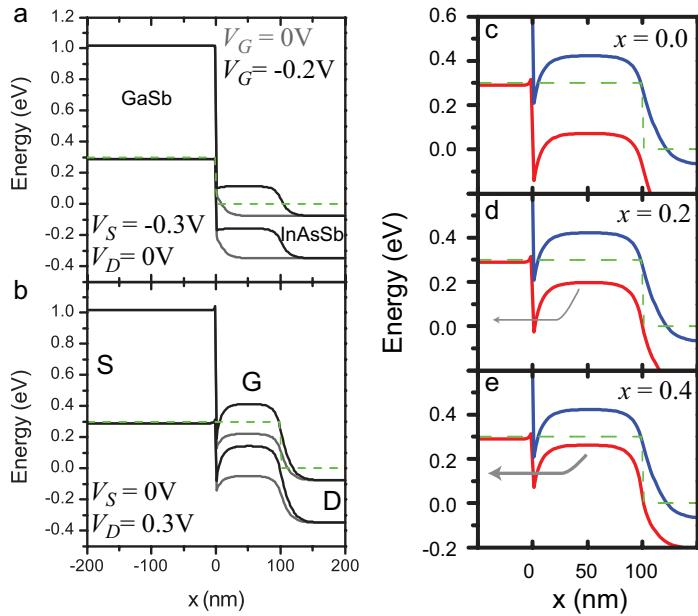
Figure 5.13: *Approximate band diagrams of GaSb/InAsSb TFETs which do not take into account carrier redistribution due to currents in the structure. Comparison of the resulting band diagram when applying an equivalent bias ( $|V_{S/D}| = 0.3$  V) to the (a) GaSb source or (b) InAsSb drain contact, respectively. Panels c-d show the effect of an increased hole leakage current due to inversion for increased Sb content in the InAsSb.*
