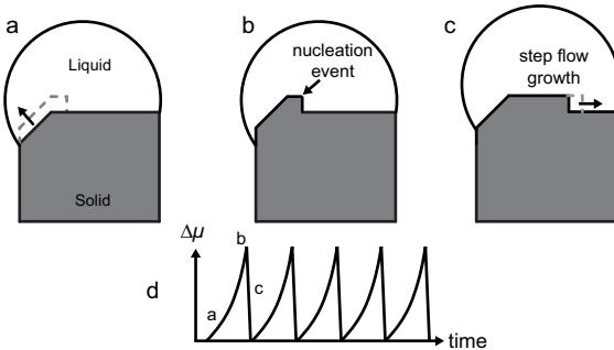
Figure 4.2: *Facet truncation driven nucleation for nanowire growth.* (a) Gradual increase in supersaturation ( $\Delta\mu$ ) which is reflected in a decrease in the size of the truncated facet until (b)  $\Delta\mu$  is sufficient for nucleation and (c) step flow growth of a new monolayer. (d) Visual representation of the supersaturation in the particle during multiple growth oscillations.
