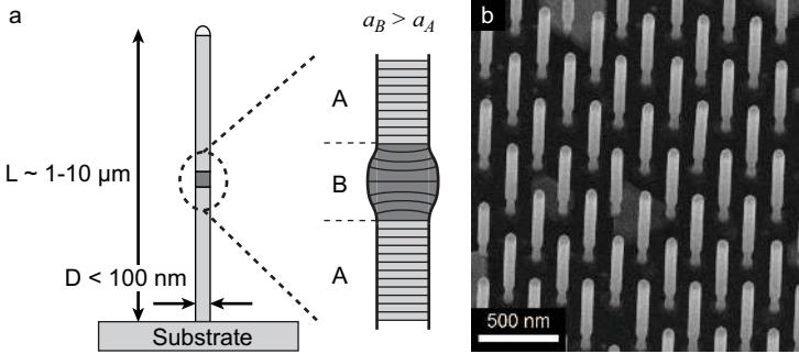
Figure 1.3: (a) *Schematic image of a nanowire of material A with a small insert of another material (B) with larger lattice parameter. The zoomed-in schematic visualizes how elastic strain may be relaxed by radial expansion in nanowires.* (b) *SEM image of an ordered InAs/InSb nanowire array grown on an InAs substrate with 7% lattice-mismatch (30° tilt angle).*
