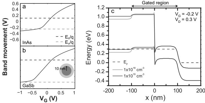
Figure 5.14: *Calculated band movement with applied gate voltage for a 20 nm-diameter (a) InAs and (b) GaSb nanowire, respectively. The gate dielectric is assumed to be 5 nm thick  $HfO_2$  ( $\epsilon_r = 25$ ). (c) GaSb/InAs<sub>0.9</sub>Sb<sub>0.1</sub> band movement with overlapping gate for two distinct p-doping levels in the GaSb source ( $N_A = 1 \times 10^{18}$  and  $1 \times 10^{19}$  cm<sup>-3</sup>) and n-doped InAsSb channel ( $N_D = 1 \times 10^{18}$  cm<sup>-3</sup>).*
