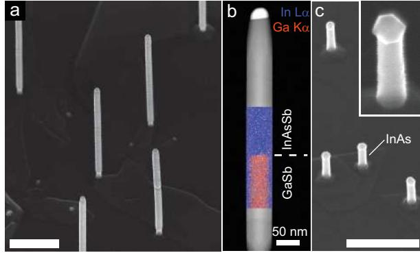
Figure 4.9: (a) SEM image of InAs-on-GaSb nanowires which have long InAs(Sb) segments grown on top of the GaSb nanowires. (b) XEDS map overlayed on a STEM image in the  $\langle 112 \rangle$  direction, revealing an abrupt Ga-to-In transition as well as a thin InAs(Sb) shell around the GaSb segment. (c) SEM image of GaSb-on-InAs nanowires. No GaSb axial segment grows at 450 °C, but the particle is faceted (inset).
