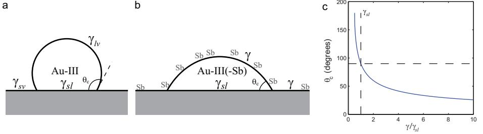
Figure 4.12: *A seed particle on a substrate (a) without and with (b) a coverage of Sb, and definition of the surface energies and contact angle. (c) Contact angle as function of the  $\gamma/\gamma_{sl}$  ratio.*
