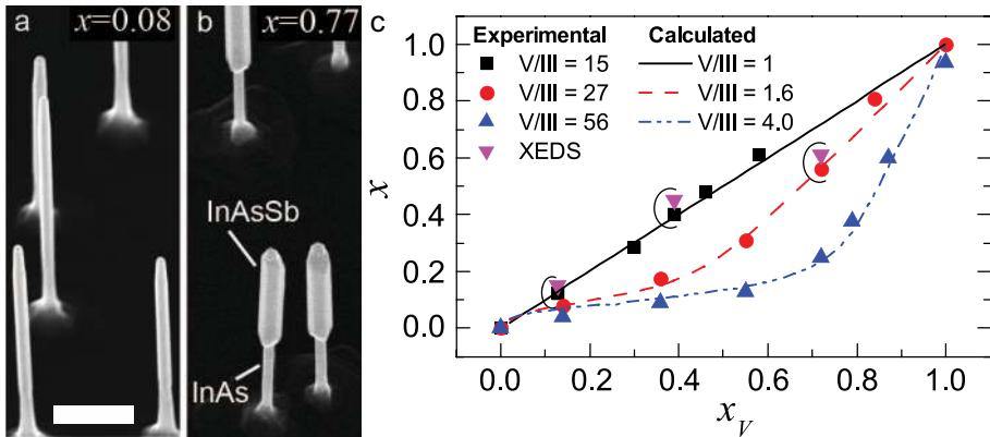
Figure 4.7: SEM images at 30° tilt angle of InAs/InAs<sub>1-x</sub>Sb<sub>x</sub> nanowires with (a)  $x = 0.08$  and (b)  $x = 0.77$  grown using the same V/III ratio and growth time. (c) InAsSb nanowire solid composition ( $x$ ) for various  $x_V$  when grown with nominal V/III ratio=15, 27, and 56. For comparison, XEDS composition measurements are also shown for a few samples. The lines are solutions of a thermodynamic calculation using only the V/III ratio as a variable parameter.
