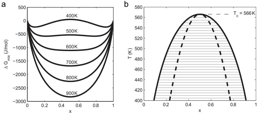
Figure 3.4: (a) The change in Gibbs free energy when mixing an  $\text{InAs}_{1-x}\text{Sb}_x$  alloy with composition  $x$ . Note the double minima developing for the lowest temperatures. These points give rise to the solid black line in (b), below which there is a miscibility gap (grey horizontal lines). The dashed lines indicate the spinoidal region in which decomposition into two separate phases is preferential.
