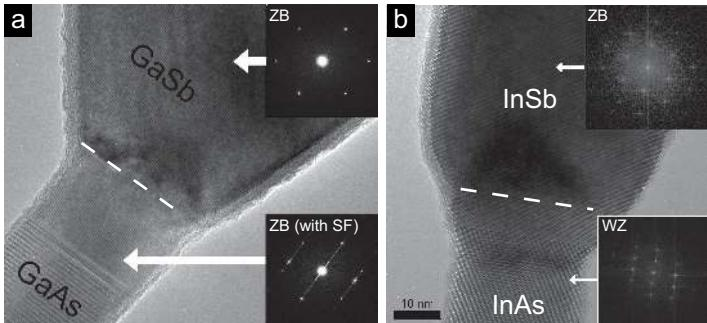
Figure 4.10: *HRTEM images of (a) GaAs/GaSb and (b) InAs/InSb nanowire heterojunctions depicting the pure ZB crystal structure of the III-Sb nanowires. The insets of (a) are the diffraction patterns for the two nanowire segments, while the insets of (b) are the Fourier transformed image of the two segments of the nanowire.*
