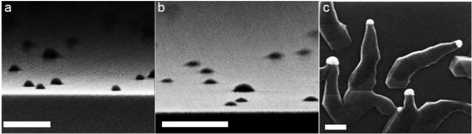
Figure 4.11: *Au particles on a GaAs(111)B substrate after annealing at 700 °C and cooling under (a) AsH<sub>3</sub> or (b) TMSb flow. Note the difference in contact angle between the two cases. (c) Au-Ga particles with GaSb trail after an attempt to nucleate GaSb nanowires directly on a GaAs(111)B substrate at 470 °C. Scale bars correspond to 200 nm.*
