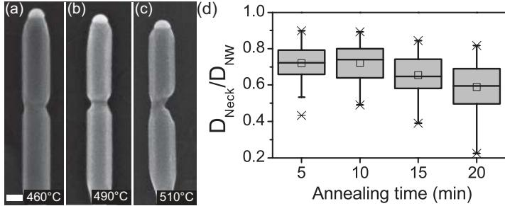
Figure 5.5: *Side-view SEM images of representative GaSb/InAsSb nanowires annealed at (a) 460, (b) 490, and (c) 510 °C for 10 min. (d) The ratio between the neck width ( $D_{\text{Neck}}$ ) and overall nanowire diameter ( $D_{\text{NW}}$ ) plotted as a function of annealing time.*
