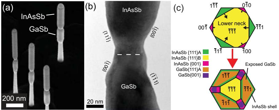
Figure 5.4: (a) SEM image at 30° tilt and (b) HRTEM image in the  $\langle 1\bar{1}0 \rangle$  zone of GaAs/GaSb/InAsSb nanowires annealed at 490 °C for 10 min. (c) Schematic visualization of the selective etching process in which  $\{111\}A$  facets are preferentially etched.
