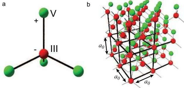
Figure 2.1: (a) Tetrahedral bonds of a III-V semiconductor indicating that the bonds are slightly ionic due to the different number of valence electrons between the group-III and group-V atoms. (b) A ZB crystal built up from cubic unit cells with a lattice parameter  $a_0$ .
