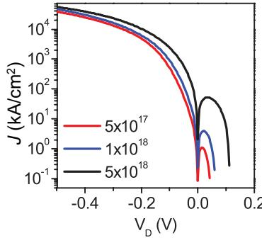
Figure 5.9: *Calculated J-V characteristics of a GaSb/InAsSb TD for three different doping levels in the GaSb segment and  $N_D^{InAsSb} = 1 \times 10^{18} \text{ cm}^{-3}$ .*
