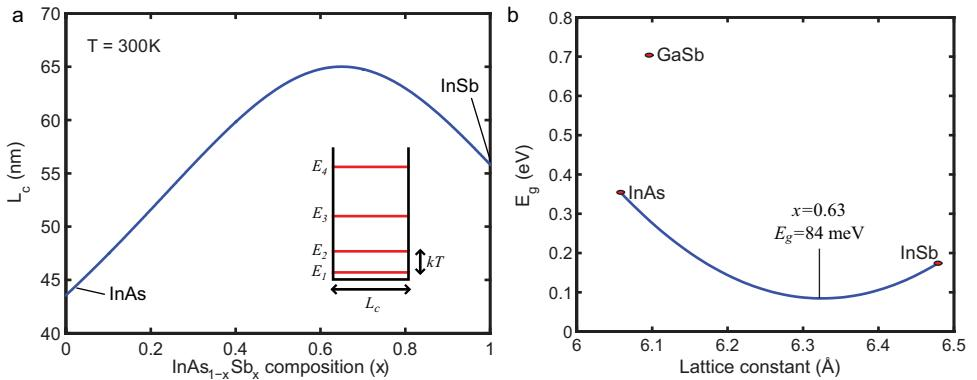
Figure 3.2: (a) Critical length in  $\text{InAs}_{1-x}\text{Sb}_x$  below which there is quantum confinement at room temperature, as a function of composition. (b) Band gap of  $\text{InAsSb}$ ,  $\text{GaSb}$ ,  $\text{InAs}$  and  $\text{InSb}$  as function of the lattice parameter.
