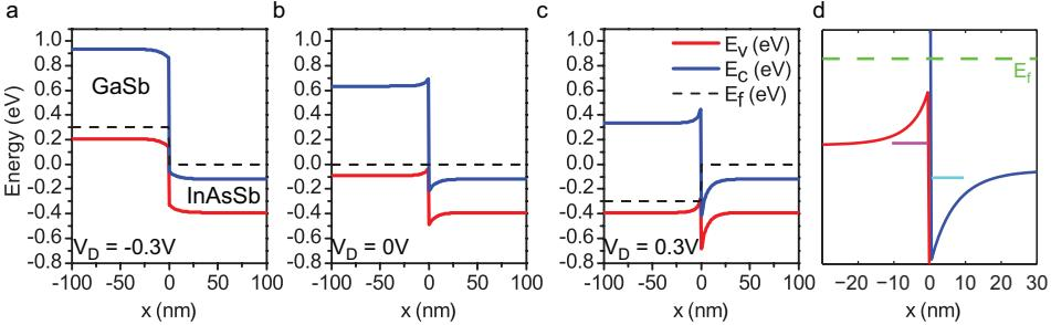
Figure 5.8: *Band diagrams of GaSb/InAs<sub>0.9</sub>Sb<sub>0.1</sub> heterojunctions obtained from a psuedo-1D Poisson solution using 2-band  $\mathbf{k} \cdot \mathbf{p}$  model to calculate the DOS, for (a)  $V_D = -0.3$  V, (b)  $V_D = 0$  V, and (c)  $V_D = 0.3$  V. (d) Close-up of the accumulation regions ( $V_D = 0$  V) including the position of the lowest subbands on either side of the heterointerface.*
