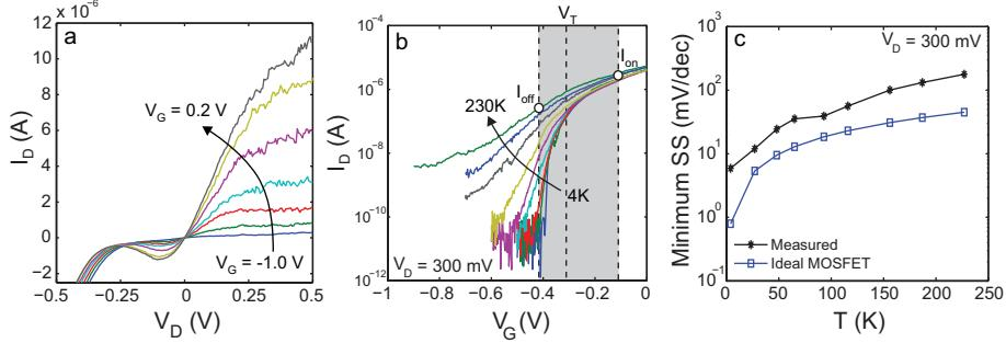
Figure 5.15: (a) Room temperature  $I$ - $V$  for various applied gate bias of a single nanowire TFET device. (b) Temperature dependence of subthreshold characteristics. The operation voltage window around  $V_T$  used to evaluate  $I_{on}$  and  $I_{off}$  at 230K is also included in this figure. (c) Temperature variation of the minimum SS for a single device, compared to the SS of an ideal MOSFET device.
