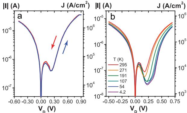
Figure 5.10: (a)  $I$ - $V$  characteristics of a processed GaSb/InAsSb single nanowire TD at room temperature. The two scans represent forward and reverse sweep directions. A clear NDR region is visible in forward bias. (b) Temperature dependence of the  $I$ - $V$  characteristics of another similar device. Note the very weak temperature dependence in reverse and small forward bias, indicating a pure tunneling current mechanism.
