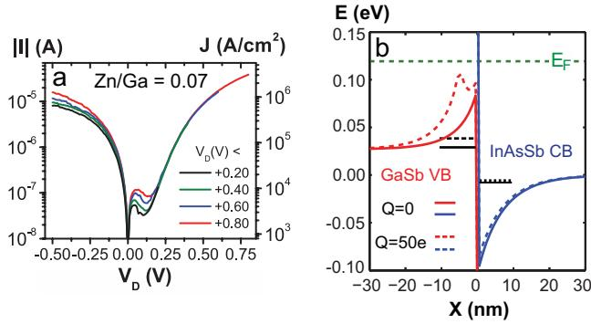
Figure 5.11: (a)  $|I|$ - $V$  sweeps on a single NW TD with various  $V_D$  magnitudes. (b) Simulation of the GaSb-InAsSb interface with and without an extra negative  $50e$  charge inserted 5 nm from the interface on the GaSb side. The black lines indicate the energy of the lowest sub-band in the wells. The extra charge broadens the GaSb well (dashed) and lifts up the light-hole sub-band.
