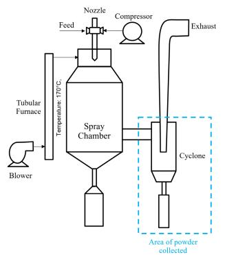
Fig. 1 Spray drying system
