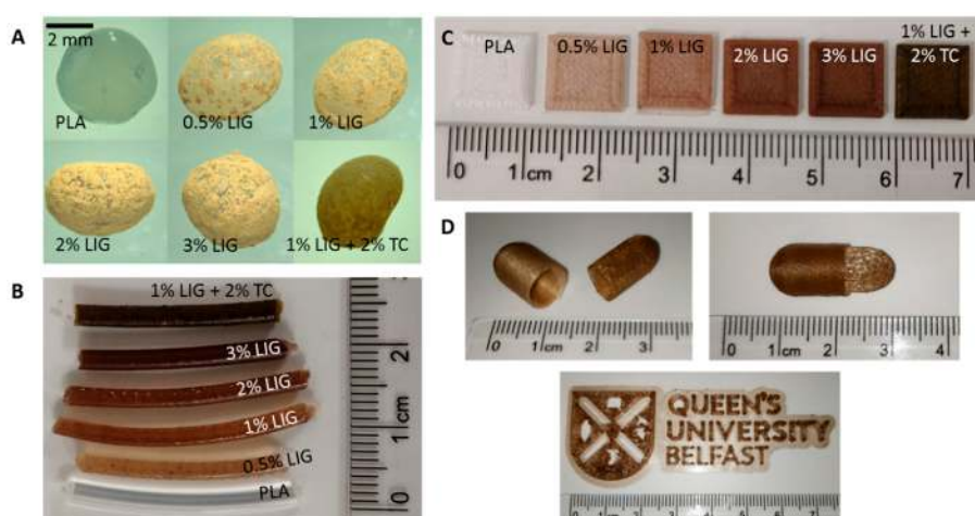
Figure 2. Photographs of: PLA and PLA coated pellets (A); LIG and TC containing PLA filaments (B); LIG and TC containing 1\text{ cm} \times 1\text{ cm} squares prepared using 3D printing (C); and different shapes printed using the filament containing 2% ( w/w ) LIG (D).
