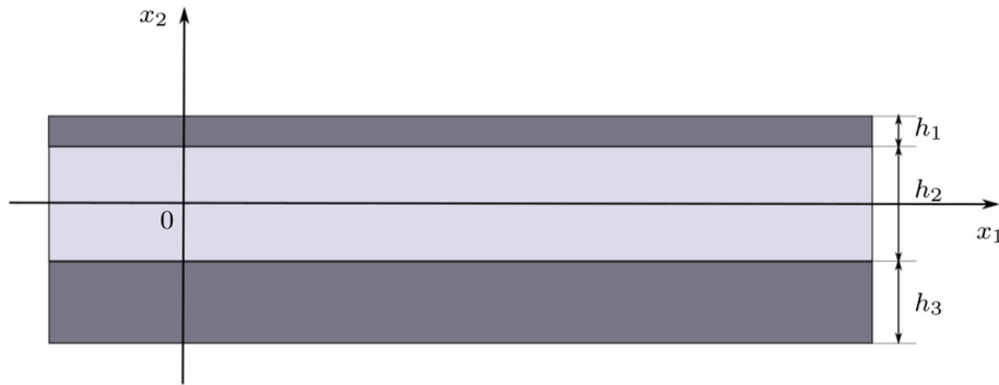
Fig. 1 A three-layered asymmetric plate
