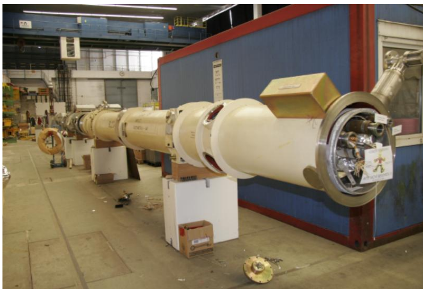
Figure 22. Setup of a HERA dipole to test the deformation method. The dipole was used as an exhibit for many years and was not foreseen as a spare for HERA.
