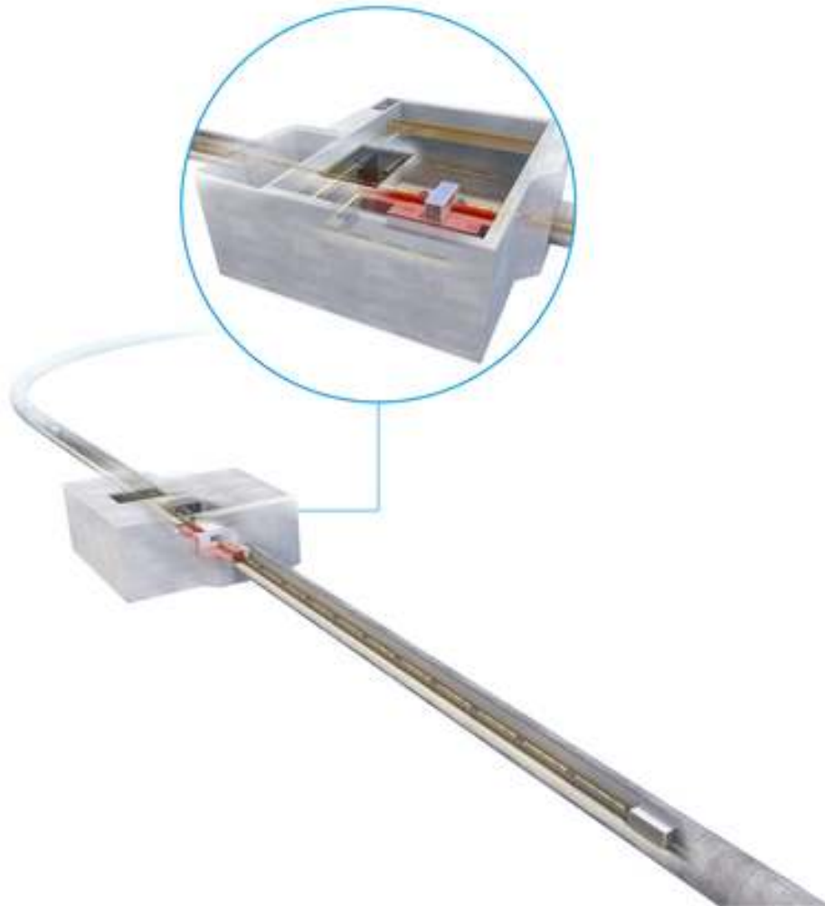
Figure 6. Artist’s view of the ALPS-IIc setup. The picture shows a straight section of the HERA tunnel equipped with 20 HERA dipoles. The middle part, accommodating the central breadboard including the “wall” is highlighted.
