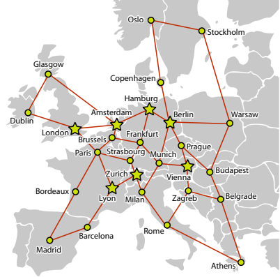
Fig. 3: NobelEU network with all possible data center (DC) locations indicated with a star symbol. Only four DCs are actually chosen in each experiment.
