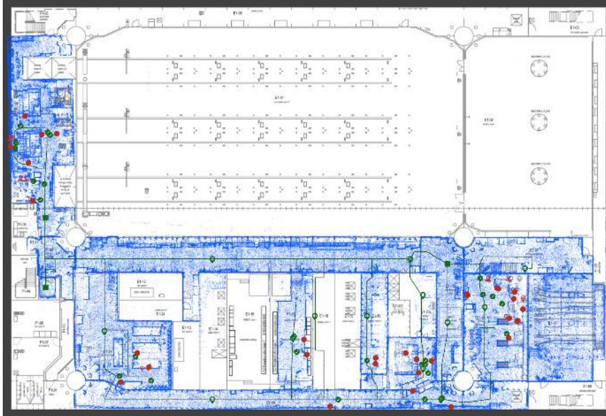
Fig. 11: The path (green) and inspection points (red) of the autonomous inspection mission is shown on the floor plan with the overlaid recorded map of the robot's sensors (blue dots).
