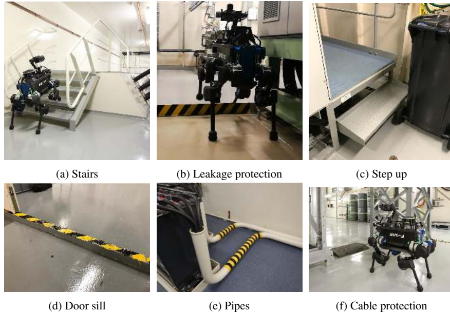
Fig. 2: Even though most of the ground is flat, various obstacles on the ground makes the locomotion of the robot difficult.
