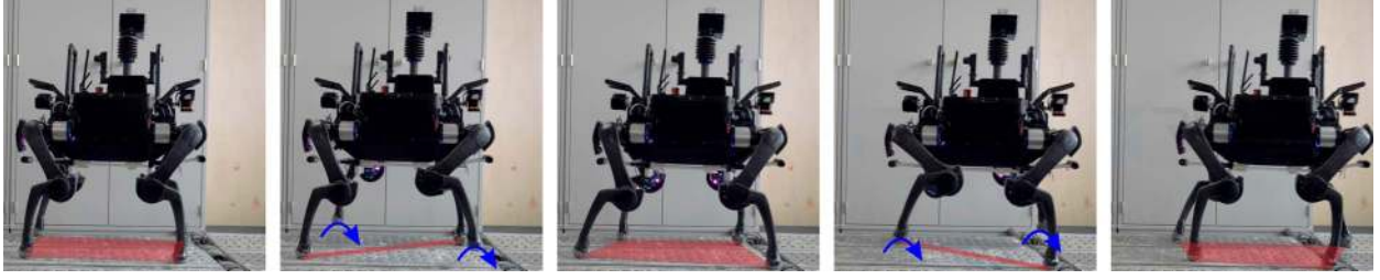
Figure 16. In most situations and for most terrains, ANYmal applies a walking trot with a duty cycle of 50%, whereby the two diagonal legs are moved together.
