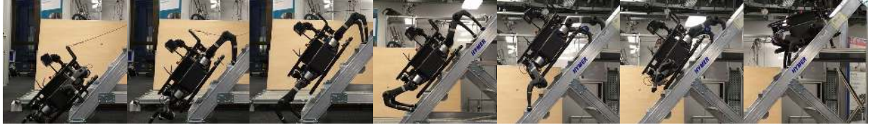
Figure 20. ANYmal can crawl up ladders of more than 50^\circ inclination. Image taken from [31].
