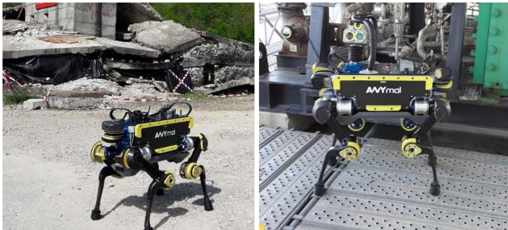
Figure 1. ANYmal, an autonomous quadrupedal robot for rough terrain operation. Depicted are two active scenarios, namely search and rescue (left) as well as industrial inspection (right).
