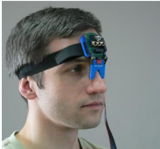
Figure 6: Saccadometer used for NoGo task (Image from Ober Consulting)
